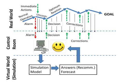
Figure 3: Principle of Real Time Physical Simulation for Emergency Management.
